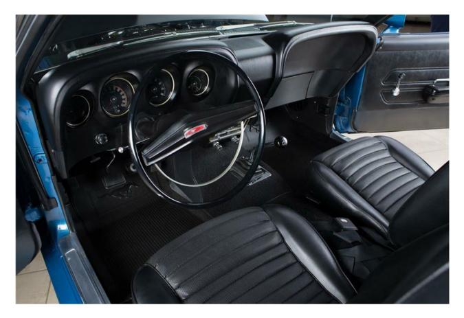
Base interiors featured the Mustang's standard gauge arrangement, which included alternator, fuel, temperature, and oil pressure gauges. Alternatively, when the option of a tachometer was selected, the Boss 302's alternator and oil pressure gauges were replaced with warning lights.
