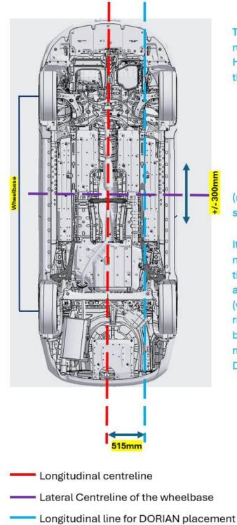
The timing transmitter (DORIAN) must be mounted on the LEFT HAND SIDE under the car with the centre of the DORIAN:
