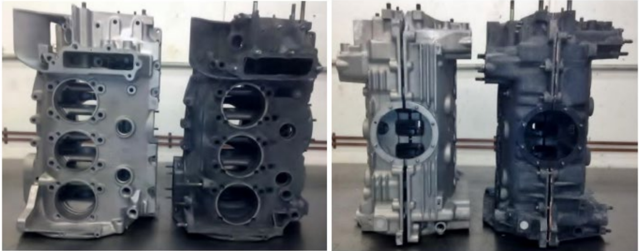
Aluminium alloy case on the left Magnesium alloy case on the Right
