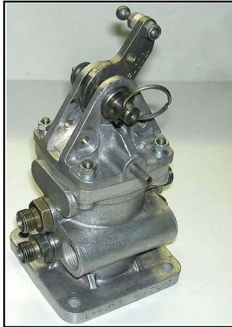
Kinsler direct linkage mixture control unit
