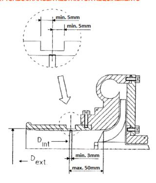
**DRAWING 2: TURBOCHARGER RESTRICTOR ALTERNATE MOUNTING**
