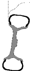
Diagram 2: Top of tyre down to flange to be within perimeter of vehicle
