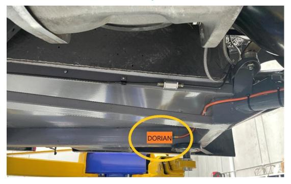
The MYLAPS transmitter must be mounted vertically on the rear panel of the front left wheel well, 75 mm from the inside corner, as shown in the diagram below.
