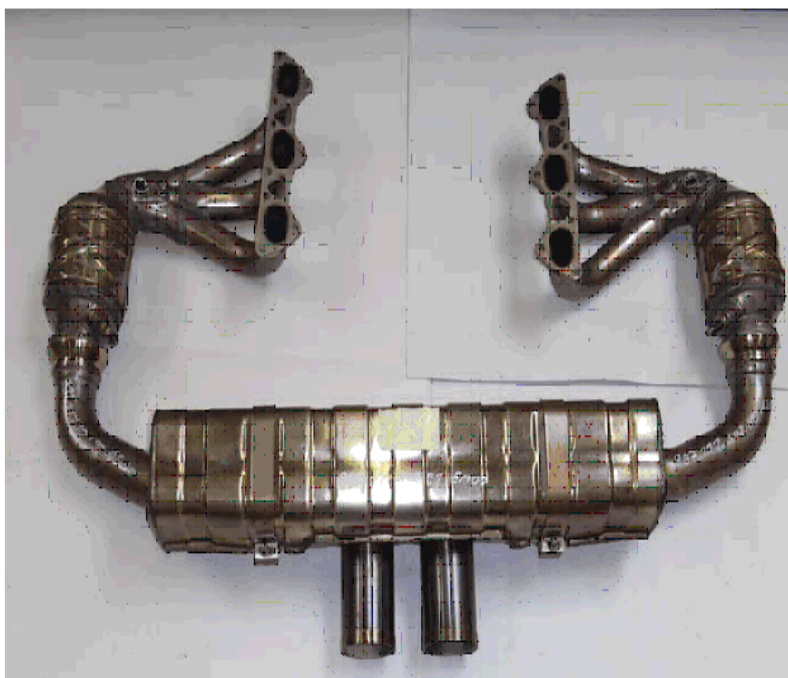
Exhaust System Nr 2 with centre rear muffler and attachments
