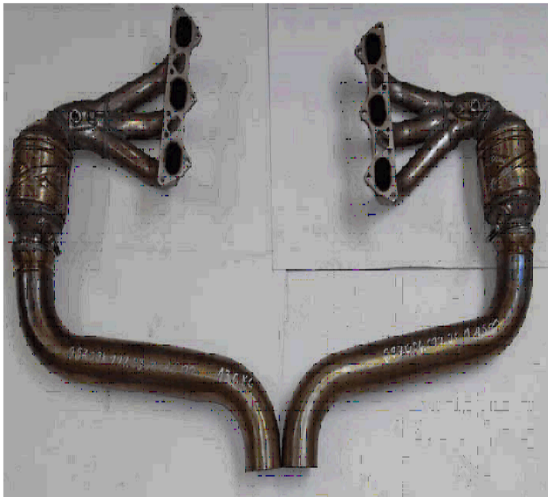
Exhaust System Nr 1 'Supercup' system
