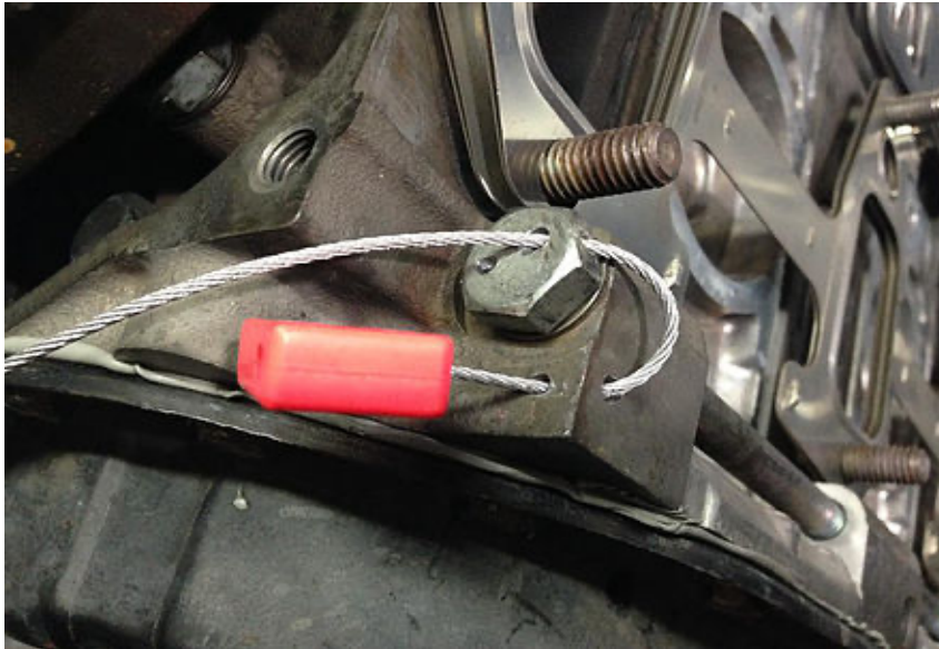
Holes to be drilled for engine seal
