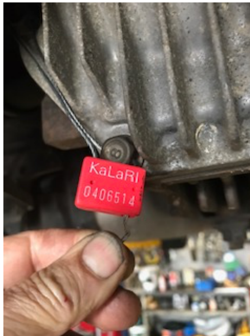
Holes to be drilled for engine seal
