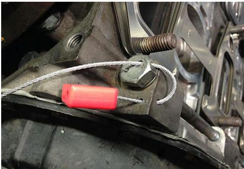
Holes to be drilled for engine seal
