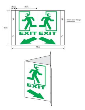
Each sign must be fixed to the fence, facing the track, at least 2 metres above track level
